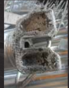
Figure 7. Not sanded cast end
