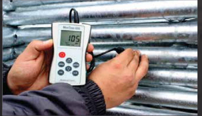
Figure 2. Measurement of the thickness of coating with a micrometer
